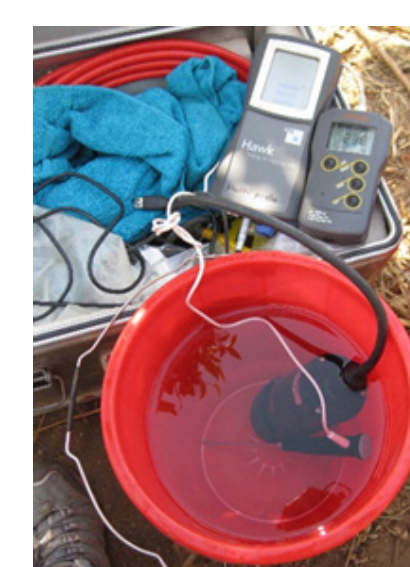
Figure 4 UviLux TLF probe and use in field (Left: NERC, 2017; Right: Ward, 2017).
